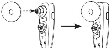
3. To wear the headset on your right ear, insert the end [A] of the head band into the rotating clip [B] on the headset until it clicks into place.
