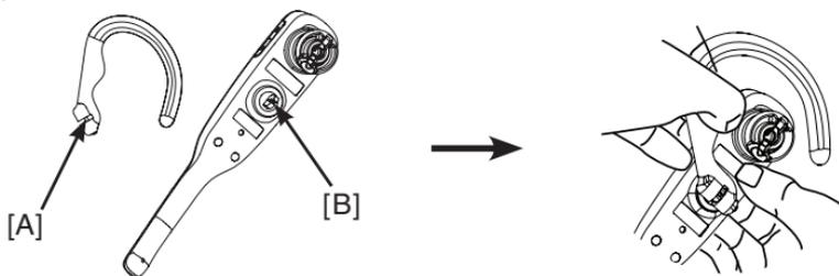
3. Hook the headset on your right ear. Adjust the angle of the headset until the microphone is pointing towards your mouth. Firmly grip the earpiece with one hand whenever adjusting the headset microphone up or down.
